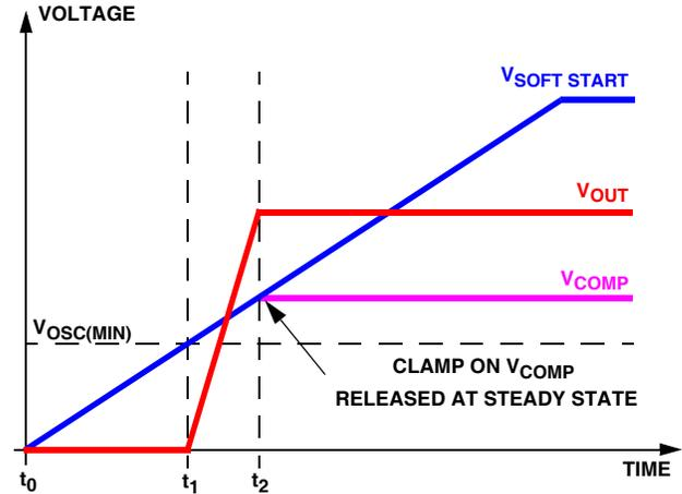
$$t_1 = \frac{C_{SS}}{I_{SS}} \cdot V_{OSC(MIN)}$$
