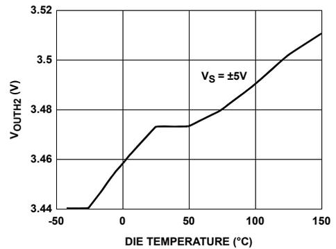
FIGURE 44. POSITIVE LOADED OUTPUT SWING vs TEMPERATURE
