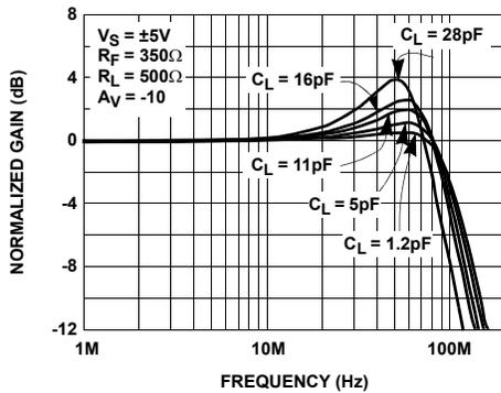
**FIGURE 15. INVERTING FREQUENCY RESPONSE FOR VARIOUS CL**
