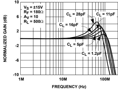
**FIGURE 14. NON-INVERTING FREQUENCY RESPONSE FOR VARIOUS CL**
