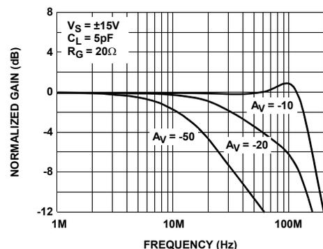
FIGURE 8. INVERTING FREQUENCY RESPONSE FOR VARIOUS  $R_F$
