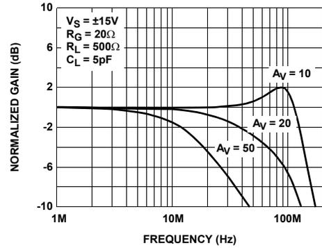
FIGURE 6. NON-INVERTING FREQUENCY RESPONSE FOR VARIOUS GAIN
