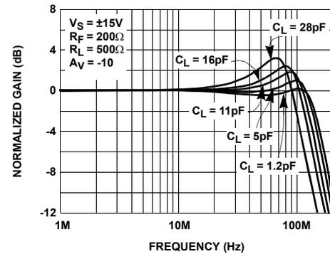
**FIGURE 16. INVERTING FREQUENCY RESPONSE FOR VARIOUS CL**
