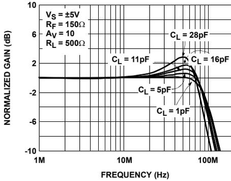
**FIGURE 13. NON-INVERTING FREQUENCY RESPONSE FOR VARIOUS CL**
