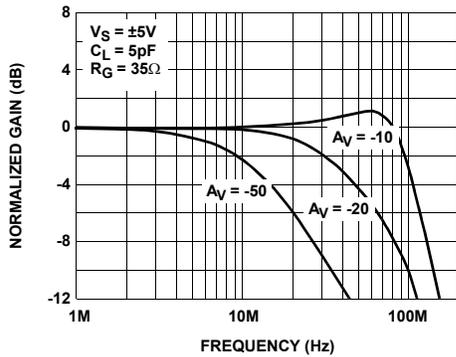
FIGURE 7. INVERTING FREQUENCY RESPONSE FOR VARIOUS GAIN
