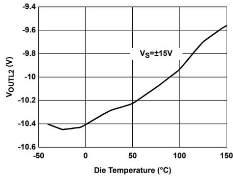
**FIGURE 47. NEGATIVE LOADED OUTPUT SWING vs TEMPERATURE**
