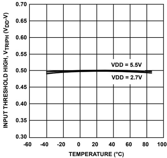
FIGURE 5. V<sub>TRIP\_H</sub> VOLTAGE
