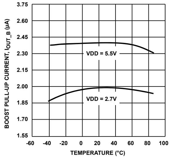
FIGURE 2. BOOST PULL-UP CURRENT, DDC PIN = V<sub>DD</sub>/2
