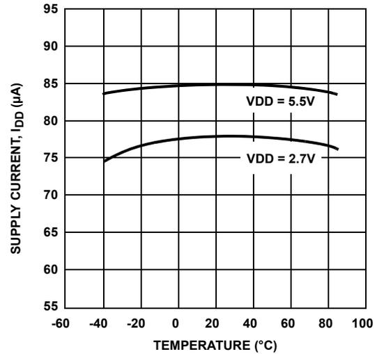
FIGURE 6. I<sub>DD</sub> CURRENT, DDC1 = DDC2 = OPEN
