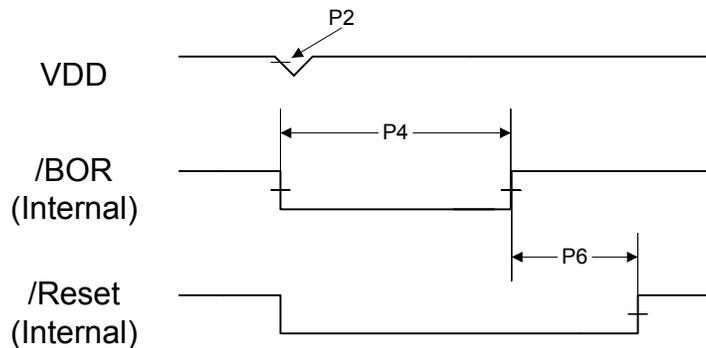
Figure 24-6. Power-On Reset and Voltage Parameters
