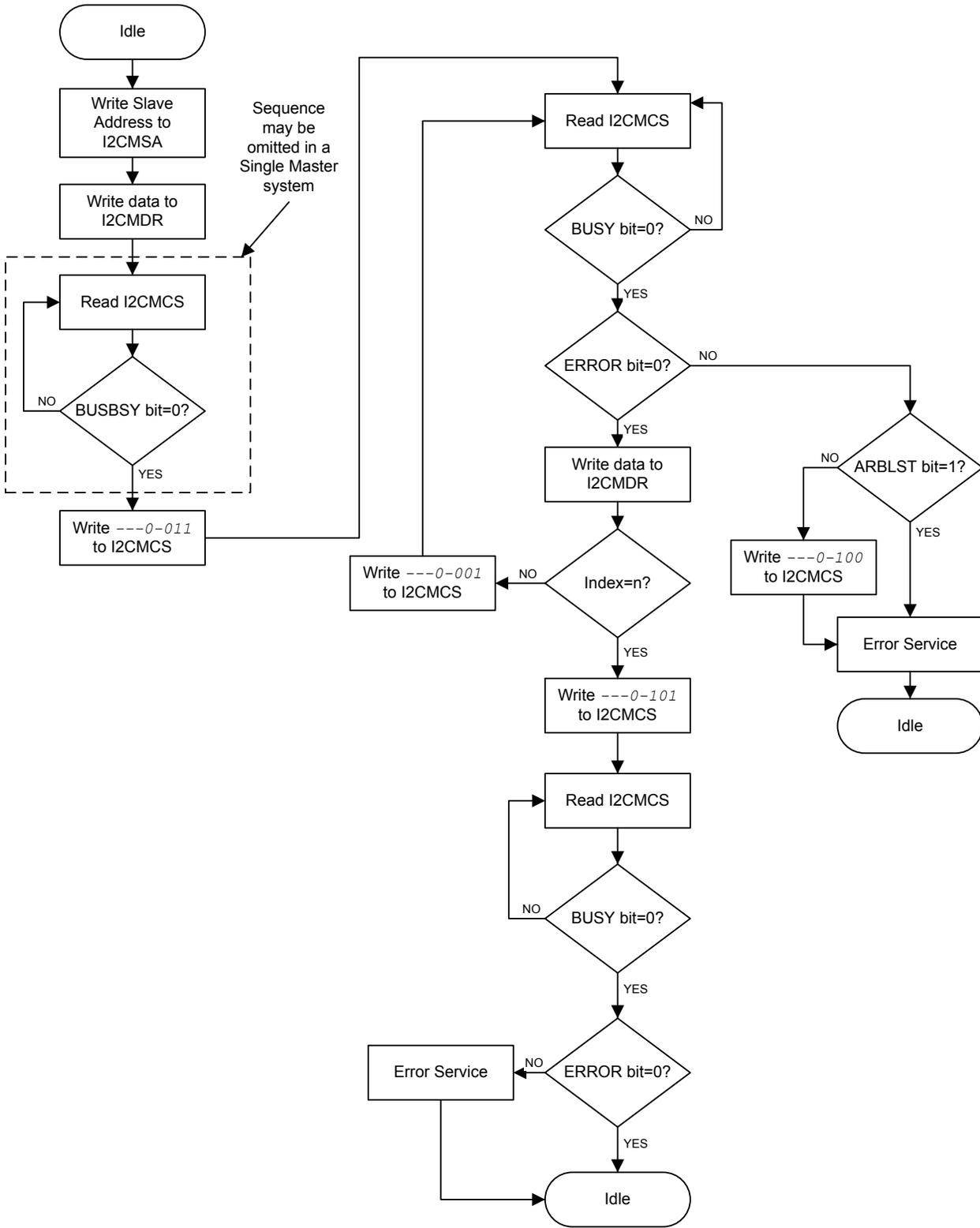
Figure 15-10. Master RECEIVE with Repeated START
