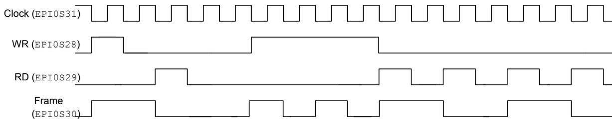
When `FRMCNT=1`, the FRAME signal transitions on the rising edge of the WR or RD strobes for every other access, see Figure 9-20 on page 474.
