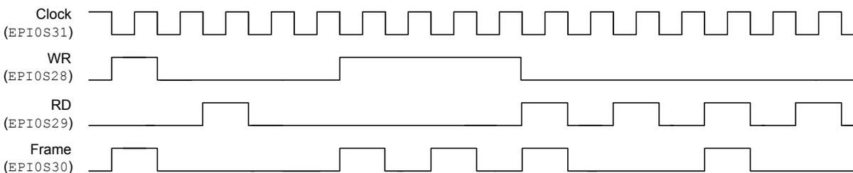
If the `FRMCNT` field is `0x2` and `FRM50` is clear, then the FRAME signal pulses high during every third access, and so on for every value of `FRMCNT`, see Figure 9-18 on page 474.
