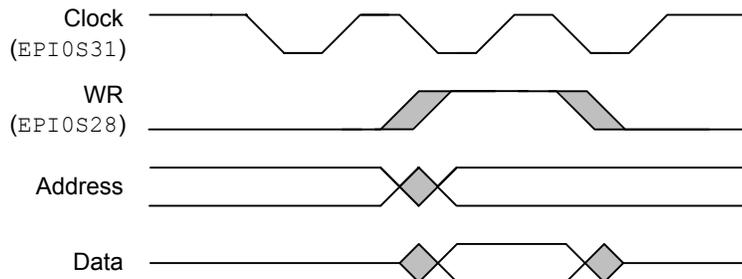
**Figure 9-24. EPI Clock Operation, CLKGATE=1, WR2CYC=1**
