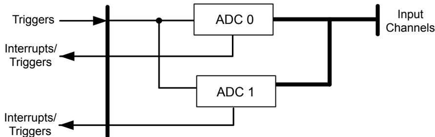
Figure 12-2 on page 592 provides details on the internal configuration of the ADC controls and data registers.
