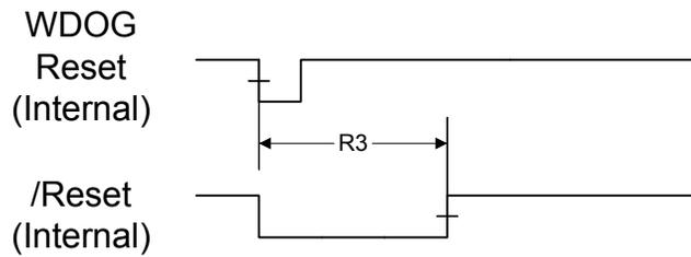
**Figure 24-10. MOSC Failure Reset Timing**
