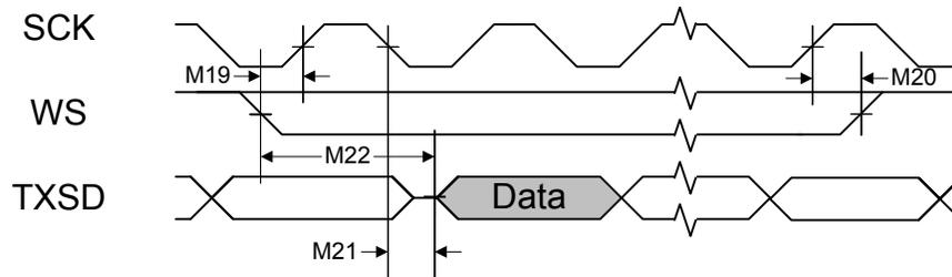
Figure 24-28. I<sup>2</sup>S Slave Mode Receive Timing
