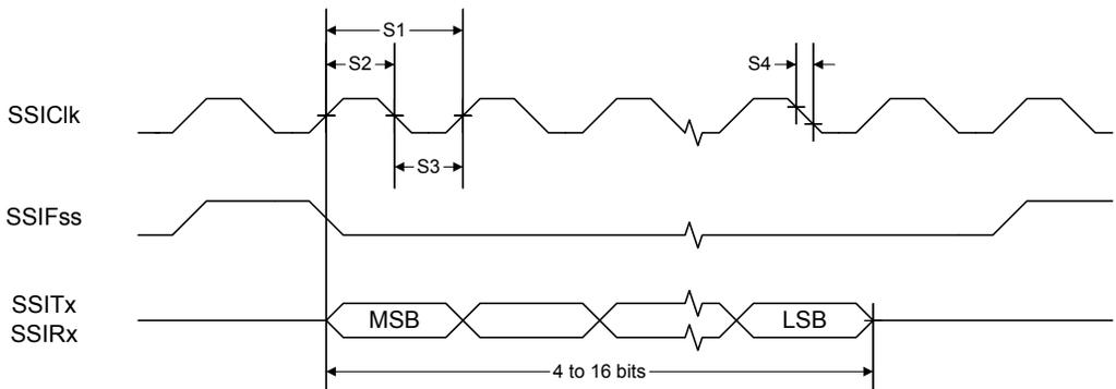
Figure 24-22. SSI Timing for MICROWIRE Frame Format (FRF=10), Single Transfer
