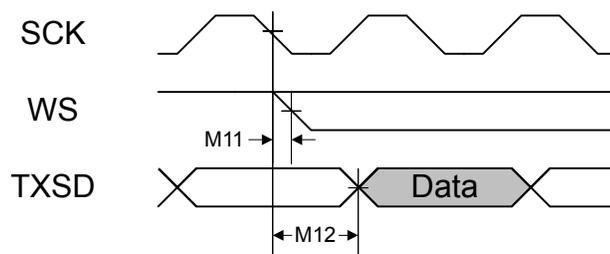
Figure 24-26. I<sup>2</sup>S Master Mode Receive Timing
