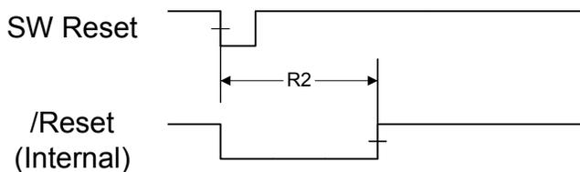
**Figure 24-9. Watchdog Reset Timing**
