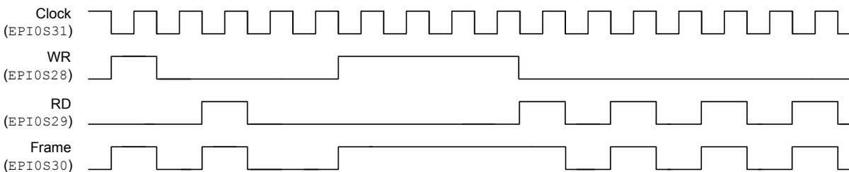
If the `FRMCNT` field is `0x1`, then the FRAME signal pulses high during every other read or write access, see Figure 9-17 on page 473.
