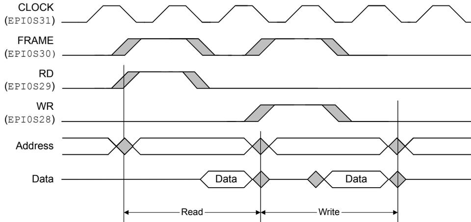
**Figure 9-15. Read Accesses, FRM50=0, FRMCNT=0, RDCYC=1**
