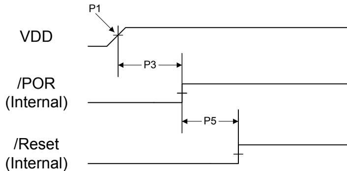
**Figure 24-5. Brown-Out Reset Timing**
