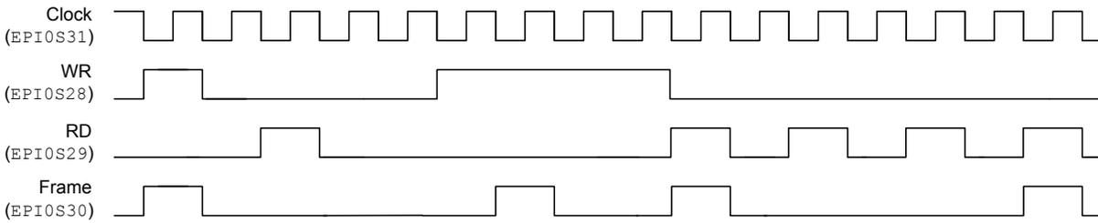
When `FRM50` is set, the FRAME signal transitions on the rising edge of either the WR or RD strobes. When `FRMCNT=0`, the FRAME signal transitions on the rising edge of WR or RD for every access, see Figure 9-19 on page 474.
