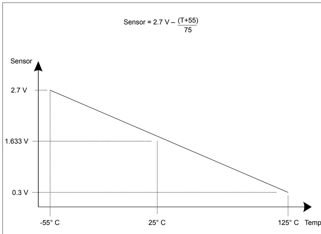
The temperature sensor reading can be sampled in a sample sequence by setting the *TSn* bit in the *ADCSCTLn* register. The temperature reading from the temperature sensor can also be given as a function of the ADC value. The following formula calculates temperature (in °C) based on the ADC reading:
