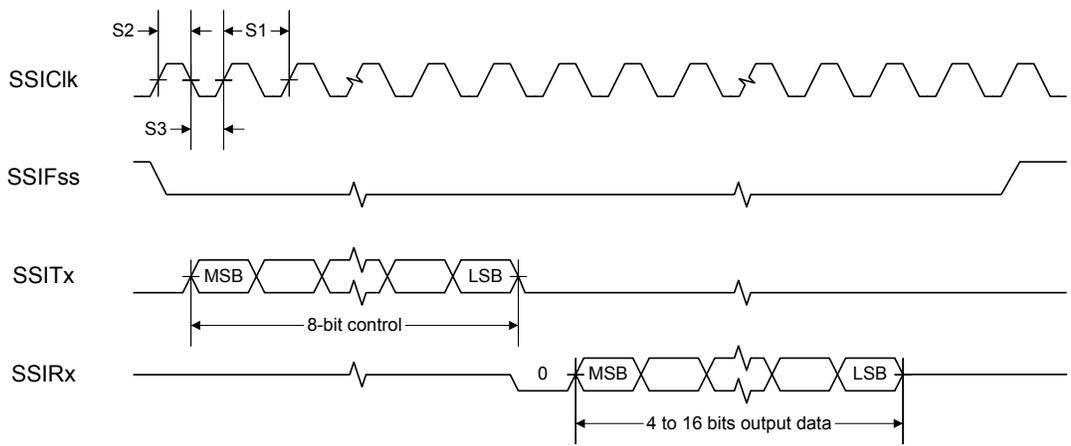
Figure 24-23. SSI Timing for SPI Frame Format (FRF=00), with SPH=1
