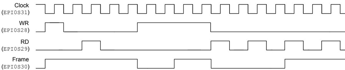
When `FRMCNT=2`, the FRAME signal transitions the rising edge of the WR or RD strobes for every third access, and so on for every value of `FRMCNT`, see Figure 9-21 on page 474.
