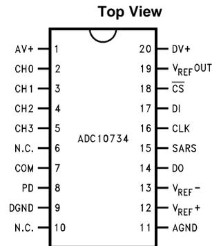
**Figure 2. ADC10734 20-Pin SOIC Package**
