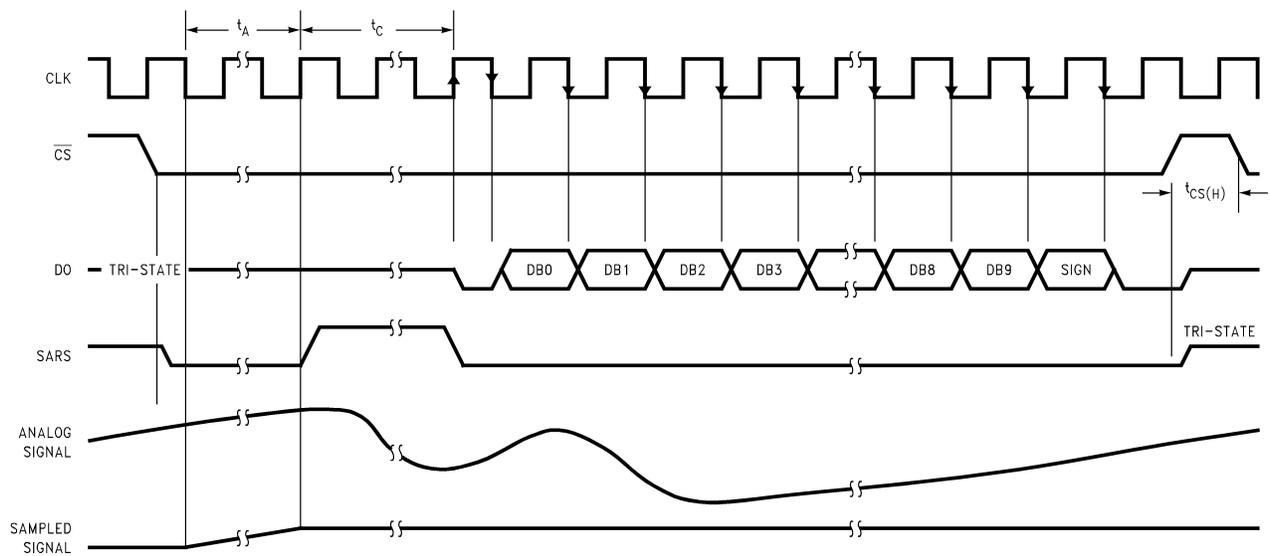
**Note:** If  $\overline{CS}$  is low during power up of the power supply voltages ( $AV^+$  and  $DV^+$ ) then  $\overline{CS}$  needs to go high for  $t_{CS(H)}$ . The data output after the first conversion is invalid.
