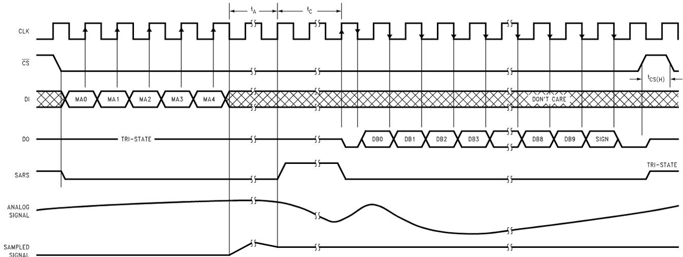
**Note:** If  $\overline{CS}$  is low during power up of the power supply voltages ( $AV^+$  and  $DV^+$ ) then  $\overline{CS}$  needs to go high for  $t_{CS(H)}$ . The data output after the first conversion is not valid.
