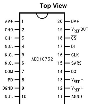
Figure 3. ADC10732 20-Pin SOIC Package
