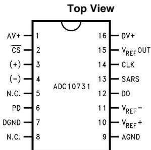
**Figure 1. ADC10731 16-Pin SOIC Package**
