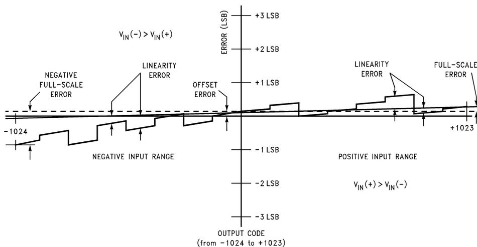
Figure 8. Simplified Error Curve vs Output Code
