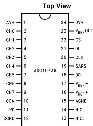
Figure 4. ADC10738 24-Pin SOIC Package
