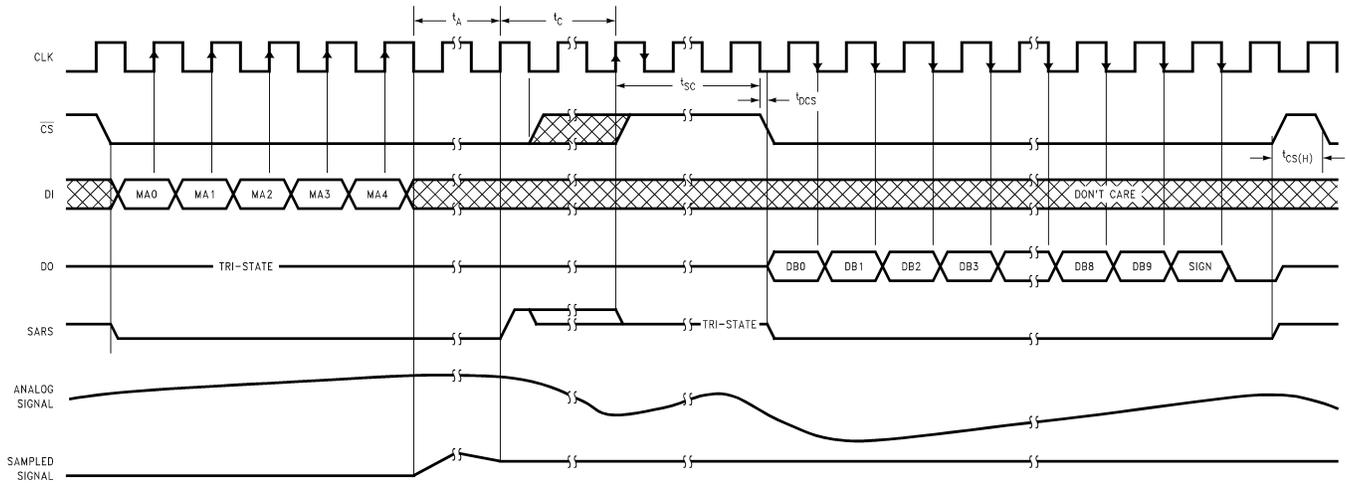
**Note:** If  $\overline{CS}$  is low during power up of the power supply voltages ( $AV^+$  and  $DV^+$ ) then  $\overline{CS}$  needs to go high for  $t_{CS(H)}$ . The data output after the first conversion is not valid.
