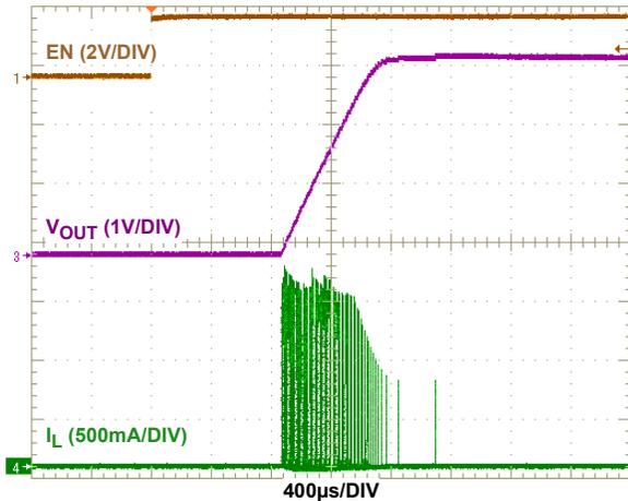
FIGURE 6. SOFT-START ( $V_{IN} = 4V$ ,  $V_{OUT} = 3.3V$ , NO LOAD)
