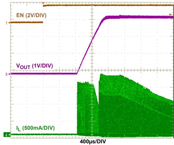
FIGURE 9. SOFT-START ( $V_{IN} = 3V$ ,  $V_{OUT} = 3.3V$ ,  $0.5A R_{LOAD}$ )
