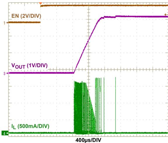
FIGURE 8. SOFT-START ( $V_{IN} = 3V$ ,  $V_{OUT} = 3.3V$ , NO LOAD)
