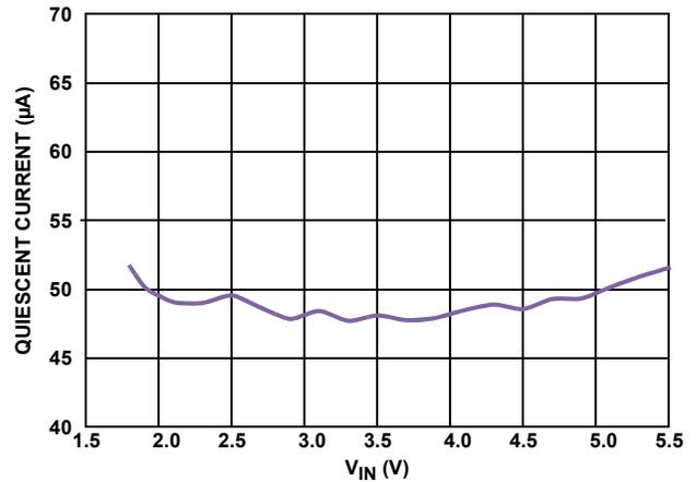
FIGURE 5. QUIESCENT CURRENT vs INPUT VOLTAGE (EN = HIGH)
