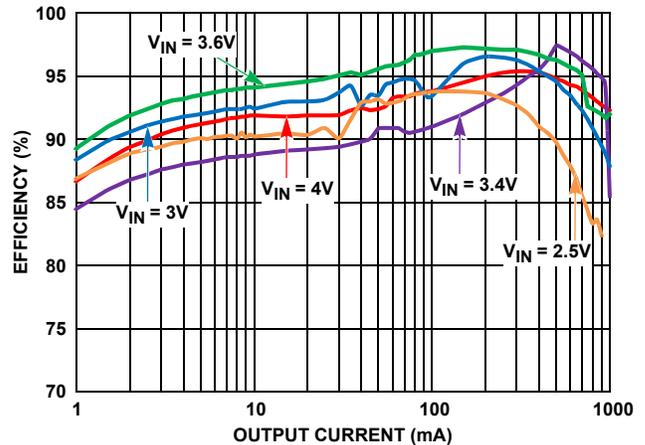
FIGURE 2. EFFICIENCY:  $V_{OUT} = 3.3V$ ,  $T_A = +25^\circ C$
