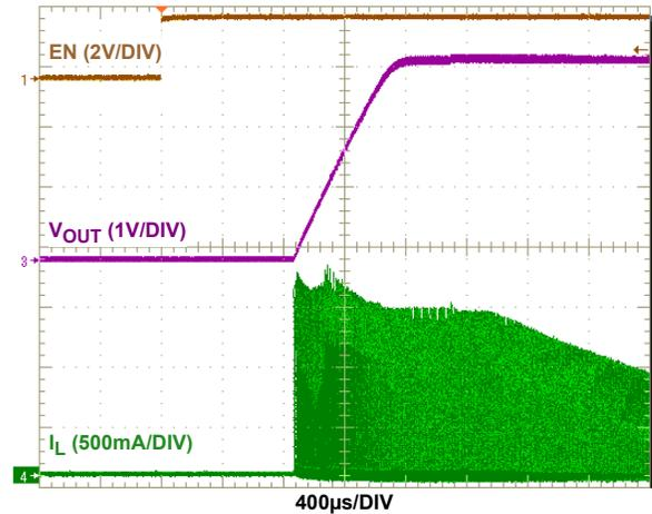
FIGURE 7. SOFT-START ( $V_{IN} = 4V$ ,  $V_{OUT} = 3.3V$ ,  $0.5A R_{LOAD}$ )
