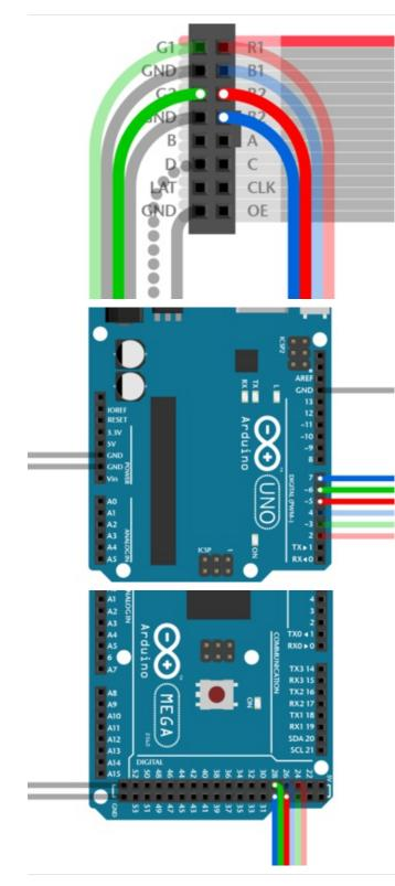
Pins **R2**, **G2** and **B2** (labeled R1, G1 and B1 on some matrices) deliver data to the **bottom half** of the display. These connect to the next three Arduino pins...
