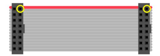
Plugged into a socket on the LED matrix, one header now faces *away* from you. If you double the cable back on itself (not a twist, but a fold)...to access a specific pin on the socket, the left and right columns are now mirrored (rows are in the same order — the red stripe provides a point of reference). You're looking "up" into the plug rather than "down" into the socket.
