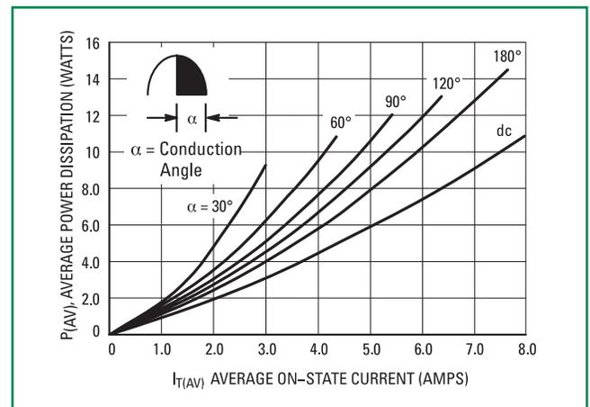
**Figure 3. On-State Characteristics**
