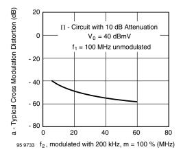
Fig. 3 - Typ. Cross Modulation Distortion vs. Frequency f<sub>2</sub>
