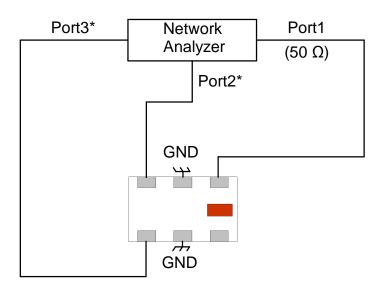
\*Impedance for ports 2 and  $3=\frac{1}{2}$  (Balanced impedance)
