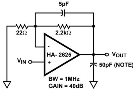
NOTE: A small load capacitance of at least 30pF (including stray capacitance) is recommended to prevent possible high frequency oscillations.
