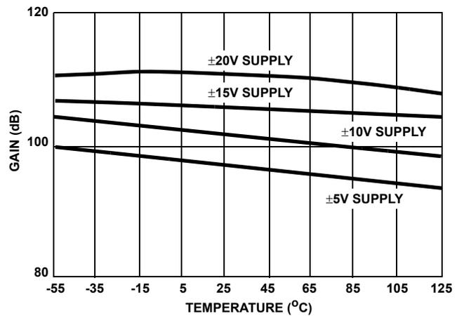
FIGURE 11. OPEN LOOP VOLTAGE GAIN vs TEMPERATURE
