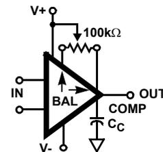
NOTE: Tested Offset Adjustment is  $|V_{OS} + 1mV|$  minimum referred to output. Typical range is ±10mV with  $R_T = 100k\Omega$ .
