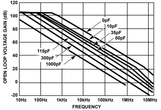
NOTE: External Compensation is required for closed loop gain < 5. If external compensation is used, also connect 100pF capacitor from output to ground.
