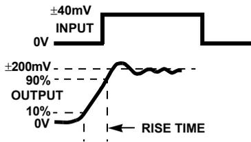
NOTE: Measured on both positive and negative transitions from 0V to +200mV and 0V to -200mV at output.
