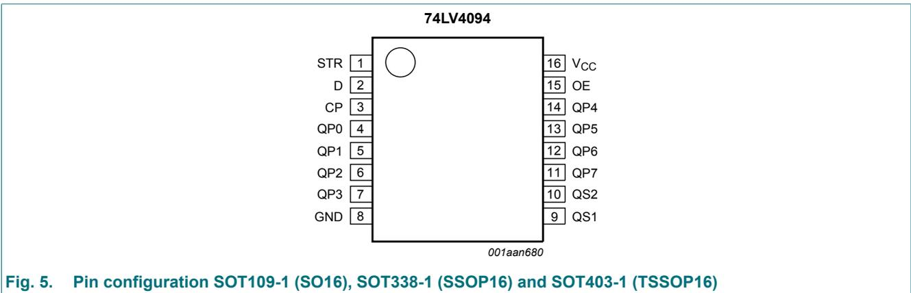
Fig. 5. Pin configuration SOT109-1 (SO16), SOT338-1 (SSOP16) and SOT403-1 (TSSOP16)
