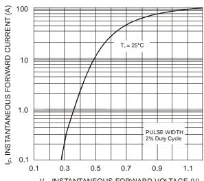
$\rm V_{F},$  INSTANTANEOUS FORWARD VOLTAGE (V) Fig. 2 Typical Forward Characteristics, Per Element
