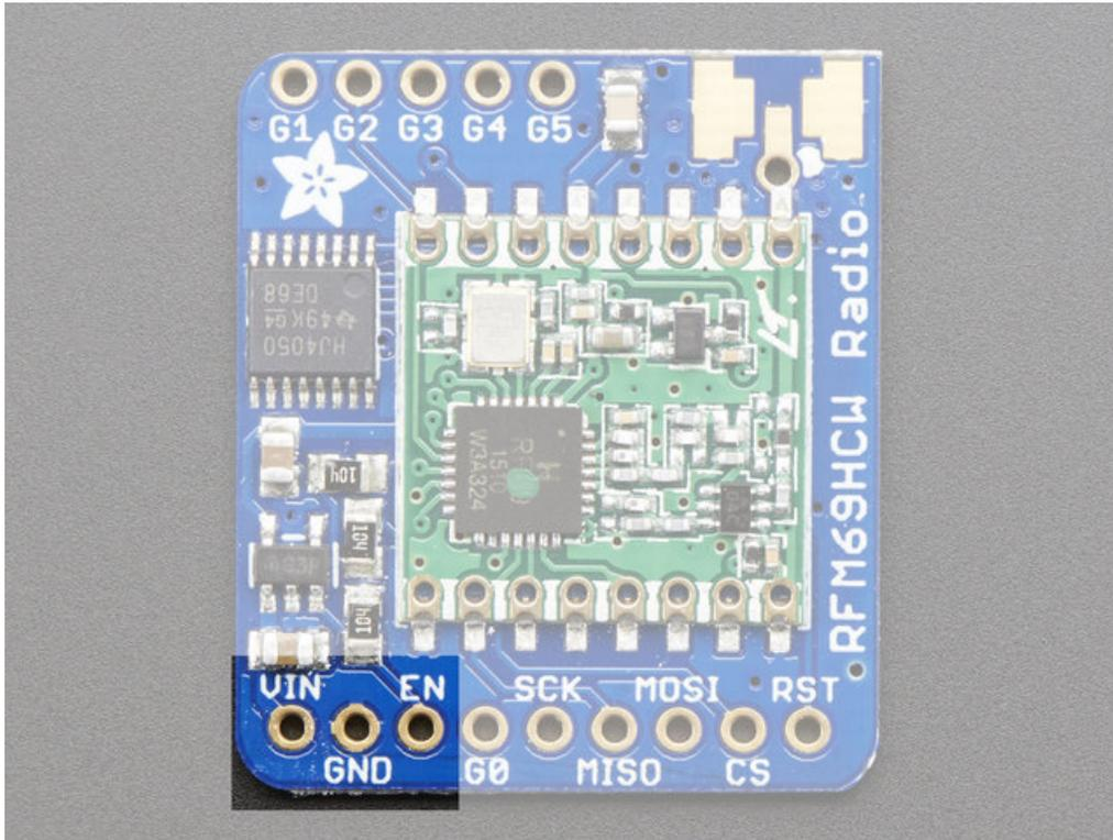
The left-most pins are used for power
