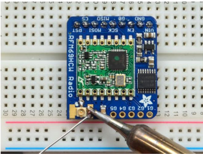
Solder in the two side pads, they are used for signal and mechanical connectivity so make sure there's plenty of solder
