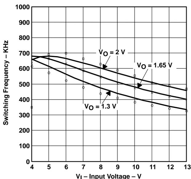
Figure 7. Theoretical (Solid) and Measured (Points) Switching Frequency
