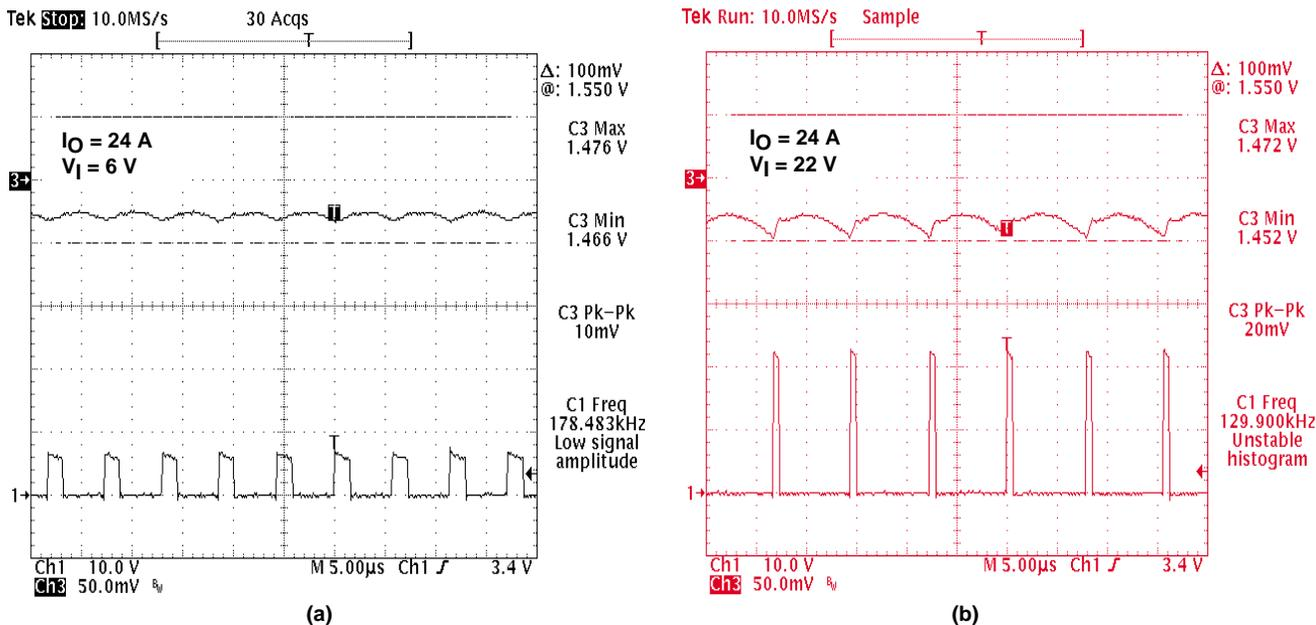
NOTE: Channel 1 = drain source voltage (10 V/div), Channel 2 = output voltage ripple (50 nV/div)
