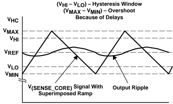
Figure 6. Hysteric Comparator Input Waveforms
