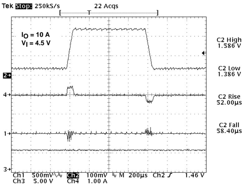
NOTE: Channel 1 = input voltage ripple, Channel 2 = output voltage, Channel 3 = VGATE signal, Channel 4 = input current.
