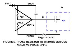
The D<sup>2</sup>-PAK, or D-PAK packaged MOSFETs, have large parasitic lead inductances and are not recommended unless a phase resistor ( $R_{PH}$ ), as shown in Figure 5, is implemented to prevent the bootstrap capacitor from overcharging, exceeding
