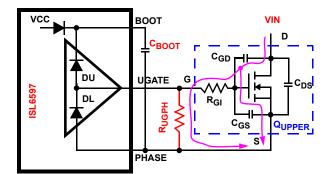
FIGURE 6. GATE TO SOURCE RESISTOR TO REDUCE UPPER MOSFET MILLER COUPLING
