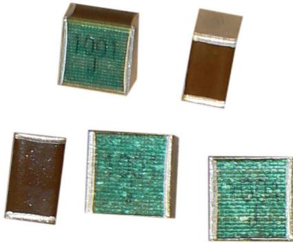
The flexible aluminum silicate dielectric eliminates cracking and permits soldering to 260 °C. These high voltage, RF capacitors need no voltage derating at temperatures up to 125 °C and voltages to 4000 Vdc. Exceptionally low ESR and superior thermal qualities set the MCH/MCHN chip capacitors apart from ordinary RF capacitors.
