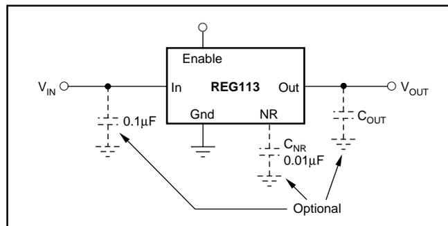
FIGURE 1. Fixed Voltage Nominal Circuit for the REG113.
