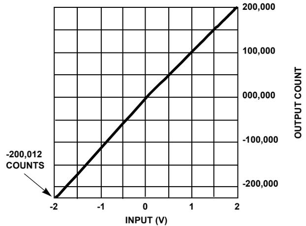
FIGURE 9. TYPICAL HI-7159A TRANSFER CHARACTERISTIC
