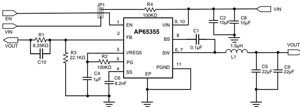
Figure 3 Typical Application of AP65355 evaluation board
