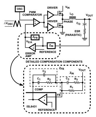
FIGURE 5. VOLTAGE-MODE BUCK CONVERTER COMPENSATION DESIGN
