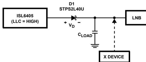
FIGURE 11. DC BACK-BIAS PROTECTION CIRCUIT
