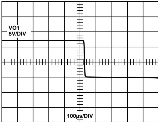
FIGURE 5. SHUTDOWN USING I<sup>2</sup>C ENABLE
