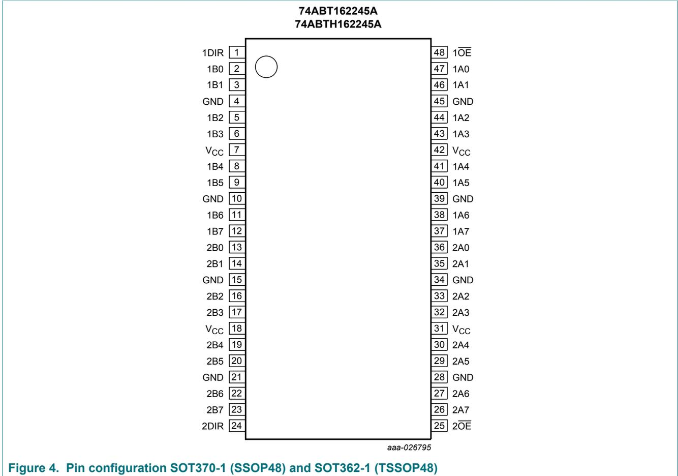
Figure 4. Pin configuration SOT370-1 (SSOP48) and SOT362-1 (TSSOP48)
