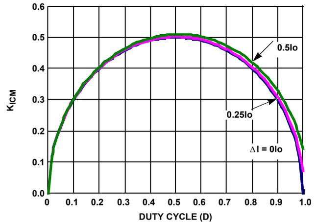
FIGURE 11. INPUT-CAPACITOR CURRENT MULTIPLIER FOR SINGLE-PHASE BUCK CONVERTER
