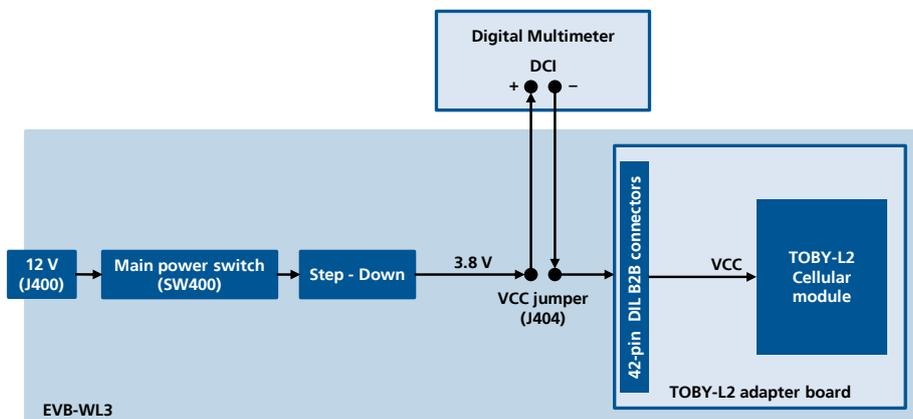
Figure 7: Block diagram of current consumption setup for TOBY-L2 modules product version "01"
