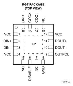
Figure 2. Pin Out of TLK4211EA in a 3 mm  $\times$  3 mm 16-Pin QFN Package
