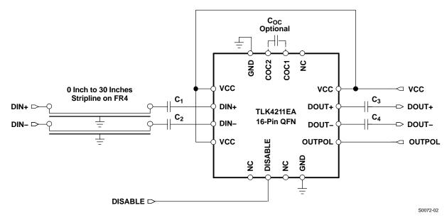
Figure 3. Basic Application Circuit With AC Coupled I/Os
