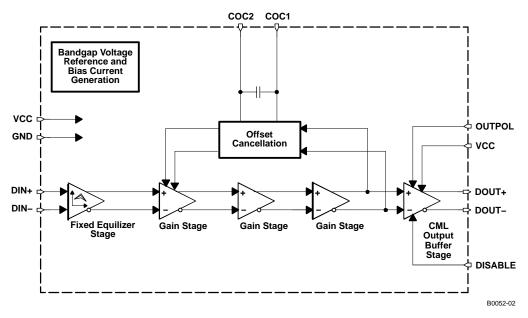
Figure 1. Simplified Block Diagram of the TLK4211EA
