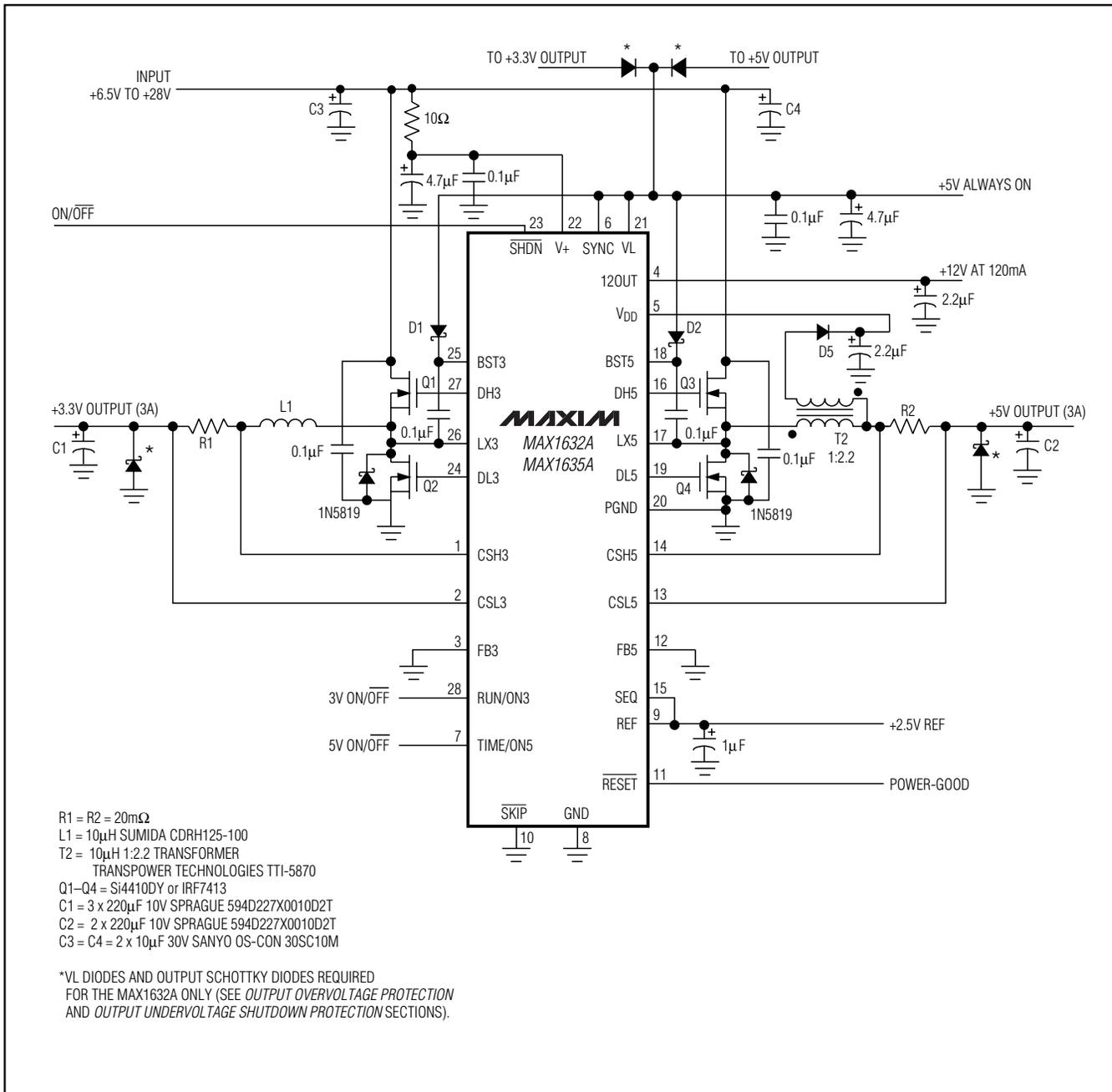
Figure 9. Triple-Output Application for High-Voltage Batteries (MAX1632A/MAX1635A)
