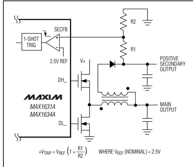
Figure 5. Adjusting the Secondary Output Voltage with SECFB
