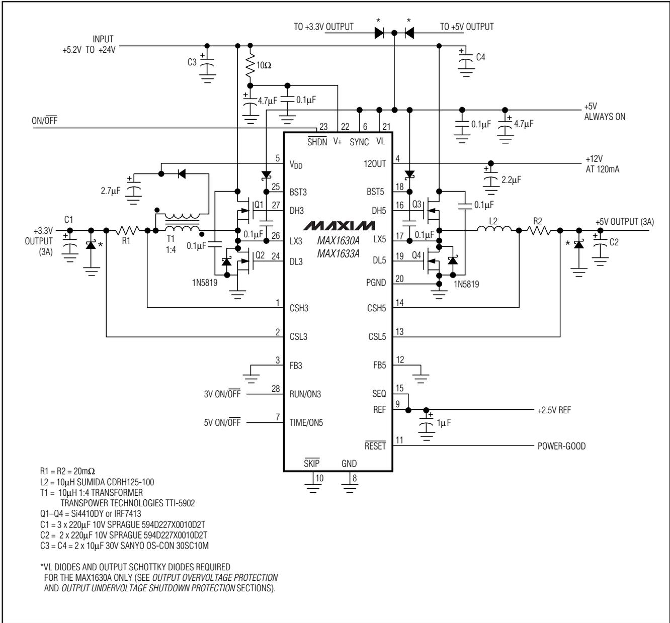
Figure 8. Triple-Output Application for Low-Voltage Batteries (MAX1630A/MAX1633A)
