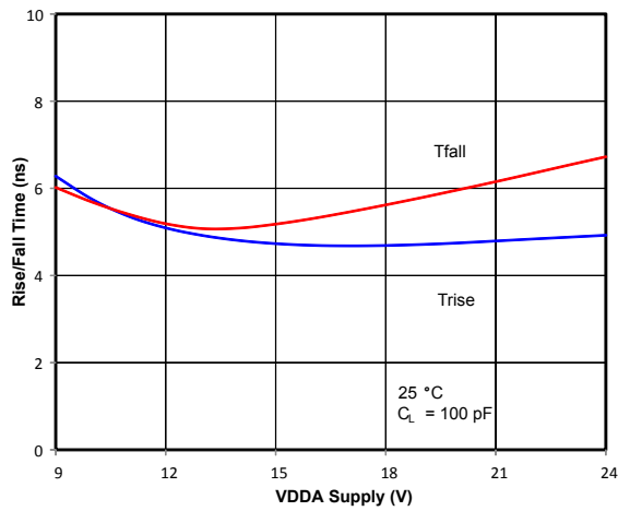
Figure 2.6. Rise/Fall Time vs. Supply Voltage
