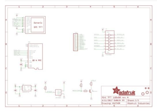
For the level shifter we use the CD74HC4050 (https://adafru.it/CgA) which has a typical propagation delay of ~10ns
