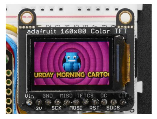
To make new bitmaps, make sure they are less than 160 by 80 pixels and save them in **24-bit BMP format**! They must be in 24-bit format, even if they are not 24-bit color as that is the easiest format for the Arduino. You can rotate images using the **setRotation()** procedure
