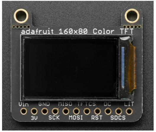
This color display uses SPI to receive image data. That means you need at least 4 pins - clock, data in, tft cs and d/c. If you'd like to have SD card usage too, add another 2 pins - data out and card cs. However, there's a couple other pins you may want to use, lets go thru them all!
