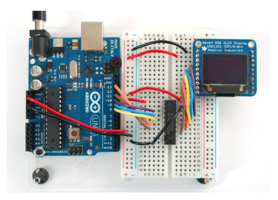
Next we'll connect the remaining 74LVC245 pins to the Arduino
