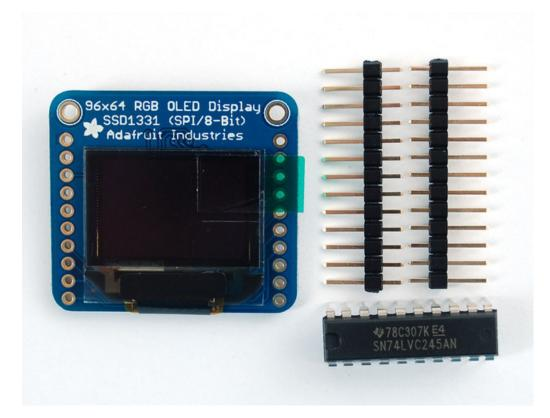
Since the OLED is 3.3V and also uses 3.3V logic, we need to use a logic shifter. We include a DIP logic shifter, the 74LVX245 with the OLED. If you're using a 3.3V logic chip, you can skip the logic shifter. Arduinos are all 5.0V so we'll be demonstrating that.
