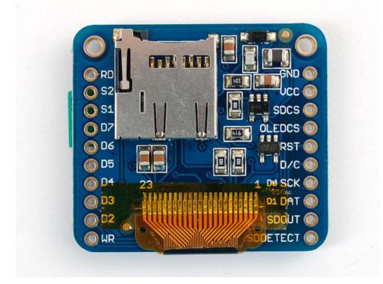
We'll have to add an extra 2 wires so we can 'select' and 'receive data' from the SD card
