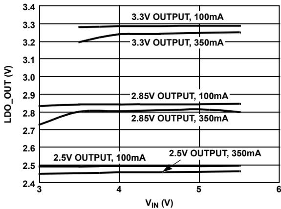
FIGURE 5. LINE REGULATION LDO\_OUT vs V<sub>IN</sub>
