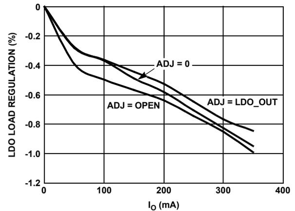
FIGURE 6. LDO LOAD REGULATION vs I<sub>O</sub>
