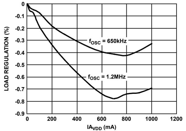
FIGURE 2. A<sub>VDD</sub> LOAD REGULATION vs I<sub>A\_VDD</sub>
