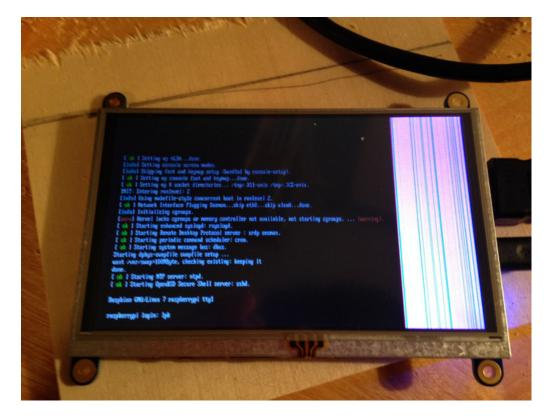
It is not broken - what is happening is you are sending 640x480 data to the monitor but since it does not have a scaler, and the display is 800x480, the remaining 160 pixels are 'not drawn' - you must set the resolution of your computer to 800x480 to get all of the pixels used! For raspberry pi, check the Config page for the correct config.txt setup for 800x480
