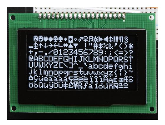
The driver chip, SSD1325 can communicate in two ways: 8-bit or SPI. Personally we think SPI is the way to go, only 4 or 5 wires are required. The OLED itself requires a 3.3V power supply and 3.3V logic levels for communication. We include a breadboard-friendly level shifter that can convert 3V or 5V down to 3V, so it can be used with 5V-logic devices like Arduino.
