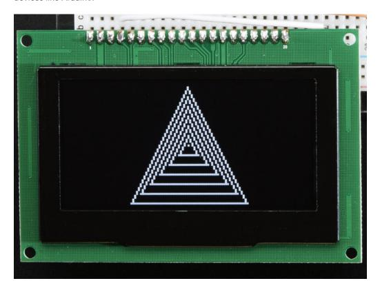
The power requirements depend a little on how much of the display is lit but on average the display uses about 50-
