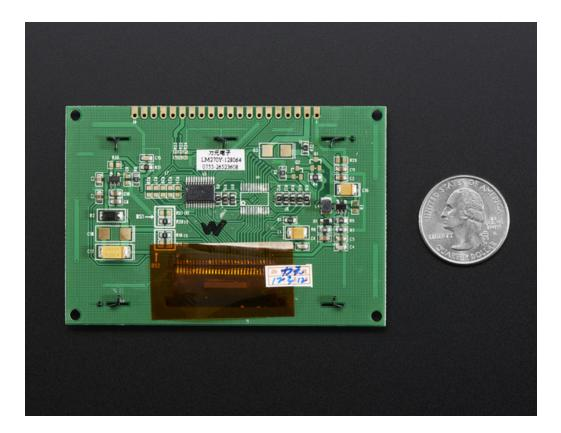
Getting started is easy! We have a detailed tutorial and example code in the form of an Arduino library for text and graphics. (https://adafru.it/iTb) You'll need a microcontroller with more than 1K of RAM since the display must be buffered. The library can print text, bitmaps, pixels, rectangles, circles and lines. It uses 1K of RAM since it needs to buffer the entire display but its very fast! The code is simple to adapt to any other microcontroller.
