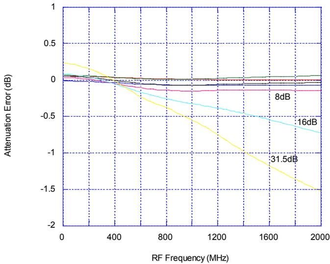
Figure 11. Attenuation Error Vs. Attenuation Setting
