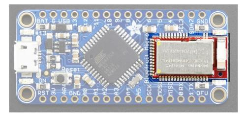
Finally there's the BLE module. This is the radio-handling part. It is an FCC/CE-certified emittermodule with a ceramic antenna. The ATmega32u4 talks to this module over SPI using our Arduino library to transmit and receive data. It is based on the nRF51822 chipset from Nordic Semiconductor.
