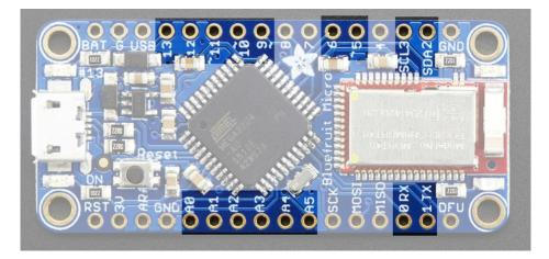
All of these pins are digital input/output pins, with 3.3V logic.Some have extra capabilities
