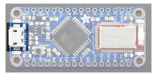
Starting from the left, there's the Micro USB connector. This is how you power and program the Bluefruit Micro. If you added on the LiPoly backpack you can also recharge the battery this way.
