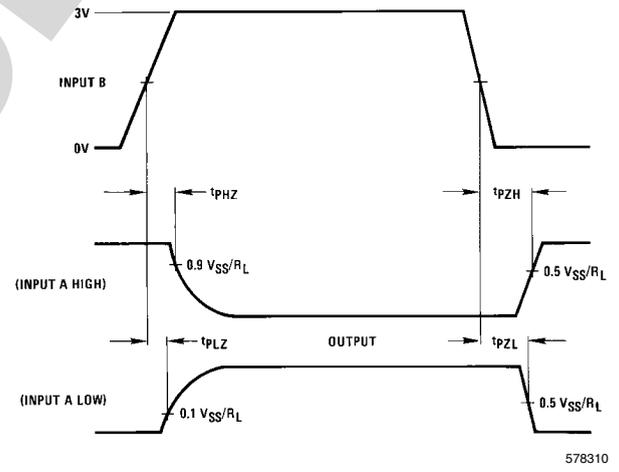
FIGURE 4. TRI-STATE Delays
