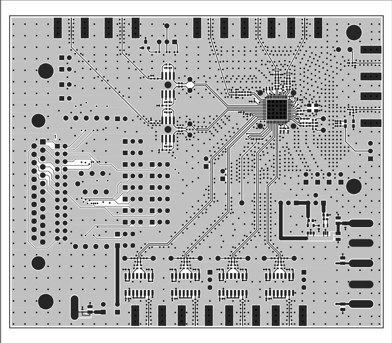
Figure 5. MAX2839AS EV Kit PCB Layout—Component Side
