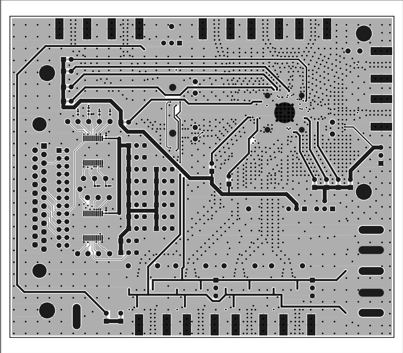
Figure 8. MAX2839AS EV Kit PCB Layout—Solder Side
