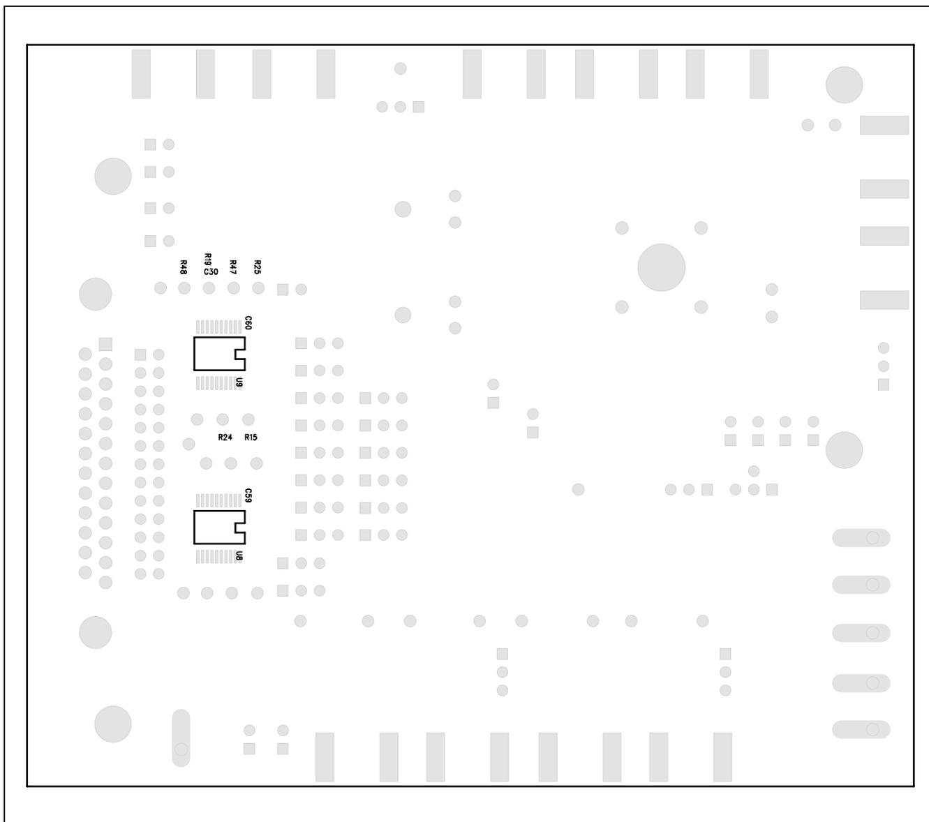
Figure 9. MAX2839AS EV Kit PCB Layout—Bottom Silkscreen
