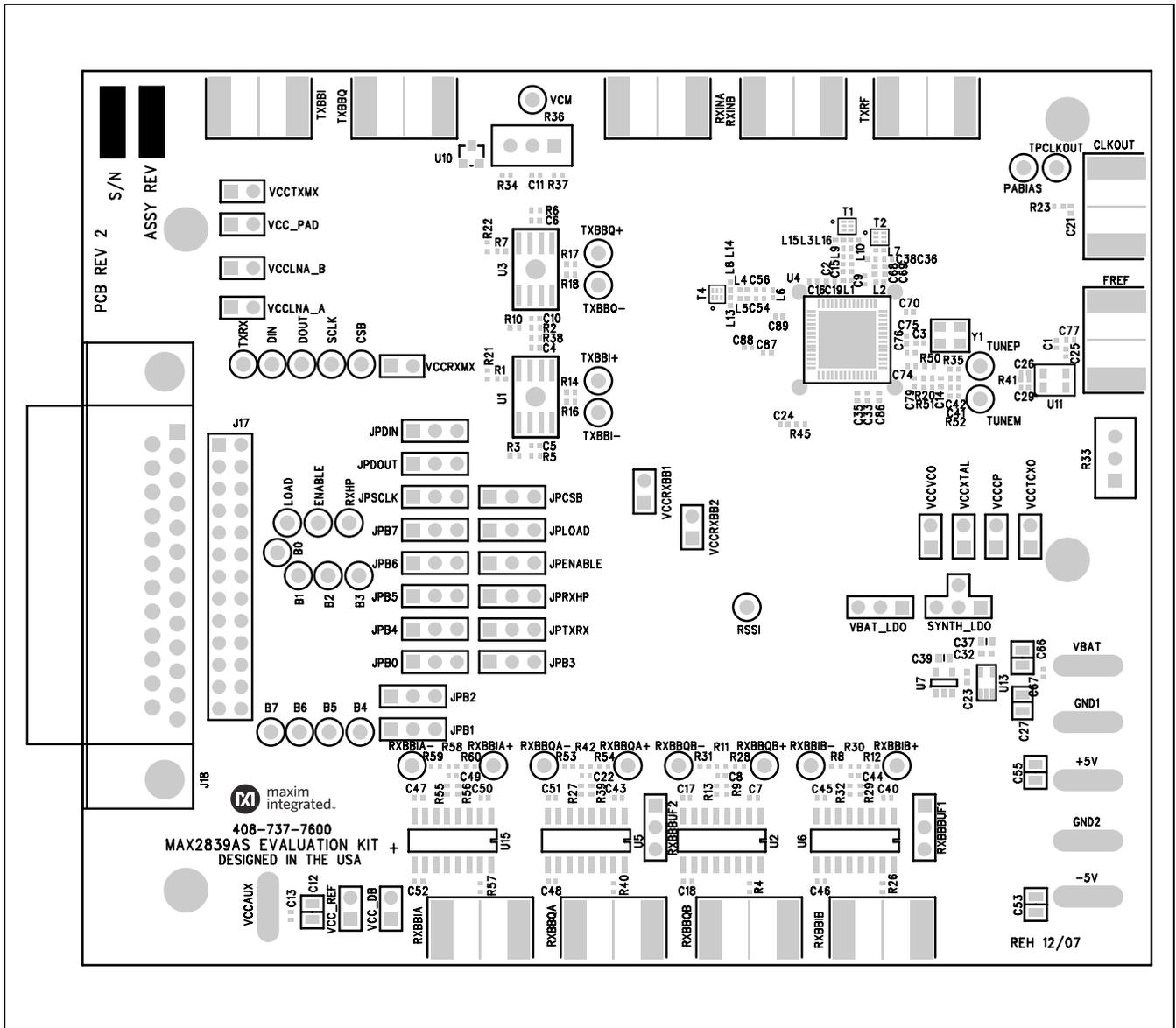
Figure 4. MAX2839AS EV Kit PCB Layout—Top Silkscreen
