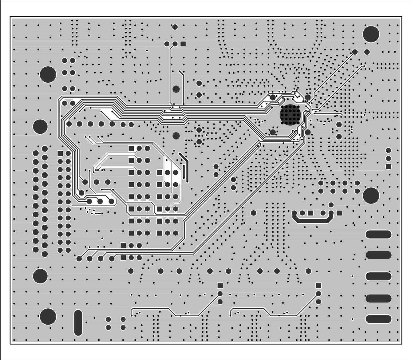
Figure 7. MAX2839AS EV Kit PCB Layout—Inner Layer 3 (Routes)
