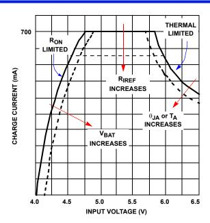
FIGURE 3. CHARGE CURRENT LIMITS IN THE CC MODE
