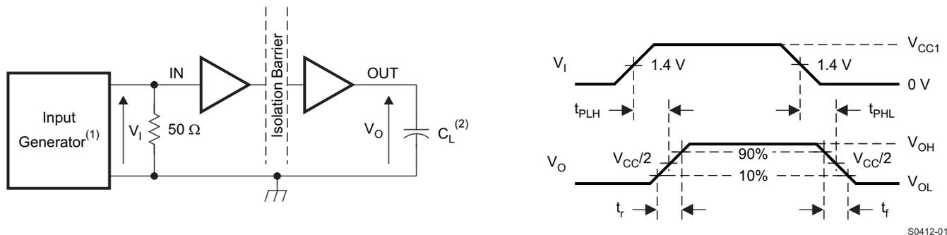
Figure 1. Switching Characteristic Test Circuit and Voltage Waveforms
