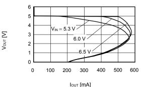
(2) Output voltage vs. Input voltage
