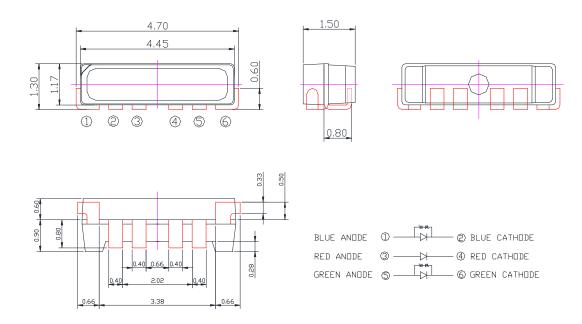
Tolerance of measurement of the dimension is  $\pm 0.1$
