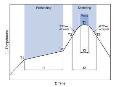
Soldering Preheating Critical zone (T3 to T4) Peak Temp. Time Temp. Time Temp. Time T1 T2 **T**4 t1 ТЗ t2 t3\* 150°C 200°C 60 to 120sec 217°C 60 to 120sec 240 to 260°C 30sec max.
