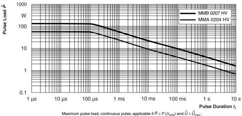
Maximum pulse load, continuous pulse; applicable if  $P \le P(S_{amb})$  and  $U \le U_{ma}$  for permissible resistance change ± (0.5 % R + 0.01  $\Omega$ )
