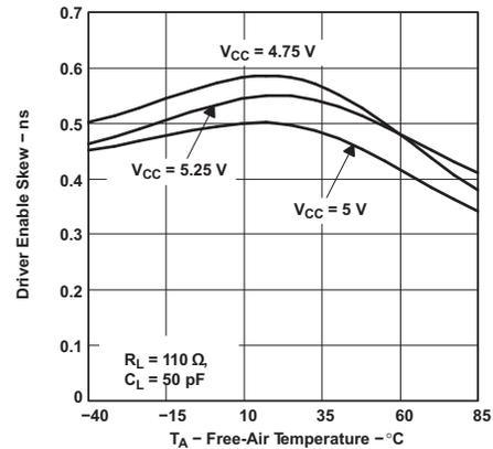
Figure 6. Driver Enable Skew vs Free-Air Temperature
