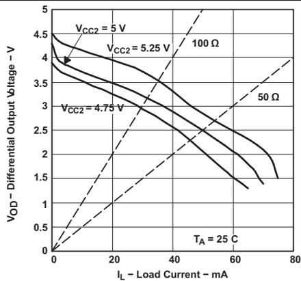
Figure 3. Differential Output Voltage vs Load Current
