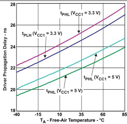
Figure 7. Driver Propagation Delay vs Free-Air Temperature
