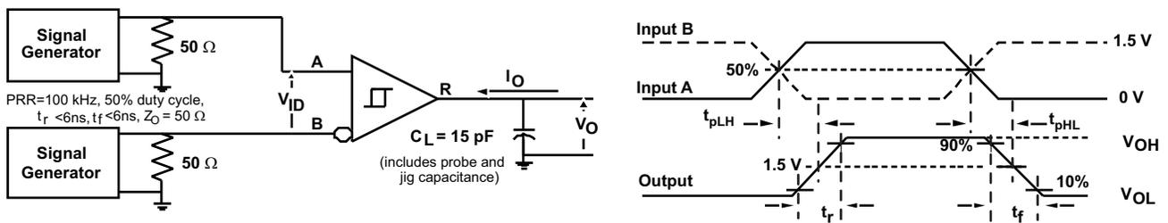
Figure 23. Receiver Switching Test Circuit and Waveforms
