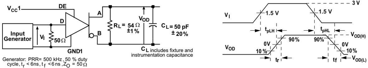
Figure 17. Driver Switching Test Circuit and Waveforms
