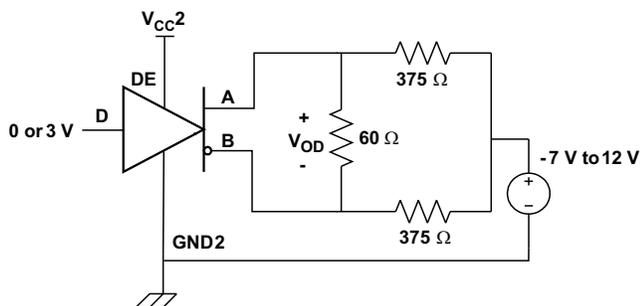
Figure 11. Driver  $V_{OD}$  with Common-mode Loading Test Circuit
