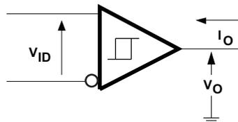
Figure 22. Receiver DC Parameter Definitions
