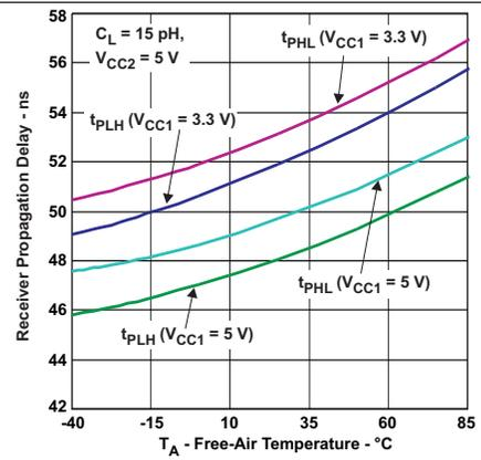
Figure 8. Receiver Propagation Delay vs Free-Air Temperature
