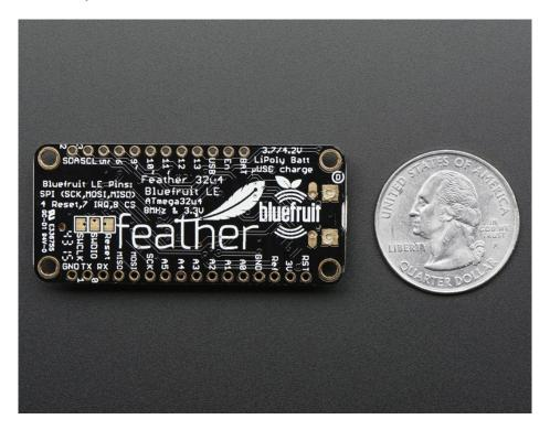
To make it easy to use for portable projects, we added a connector for any of our 3.7V Lithium polymer batteries and built in battery charging. You don't need a battery, it will run just fine straight from the micro USB connector. But, if you do have a battery, you can take it on the go, then plug in the USB to recharge. The Feather will automatically switch over to USB power when its available. We also tied the battery thru a divider to an analog pin, so you can measure and
