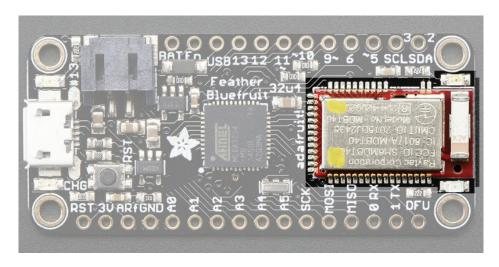
Since not all pins can be brought out to breakouts, due to the small size of the Feather, we use these to control the BLF module
