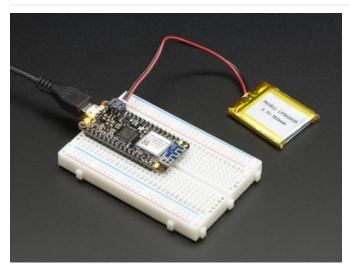
The first option is soldering in plain male headers, this lets you plug in the Feather into a solderless breadboard
