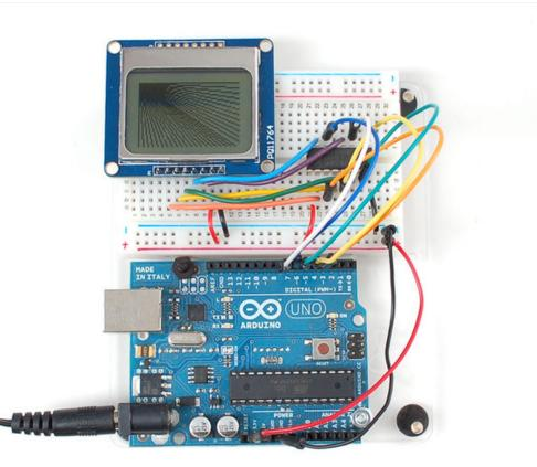
You can save some pins by connecting the CS pin to **ground** (this means you cant reuse the LCD's pins between screen updates but maybe thats OK. You can also connect the **RST** pin to the Arduino **reset** so that it will reset the screen automatically.
