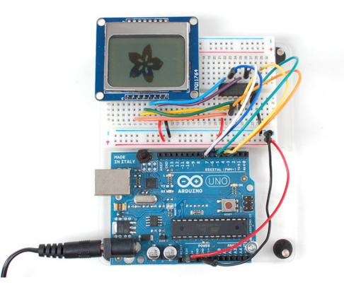
You can control the backlight, its much brighter when you connect the backlight pin to 5V (you don't need a level shifter if you are using a Nokia display from Adafruit). You can control the backlight using an Arduino pin since there is a transistor on the board.
