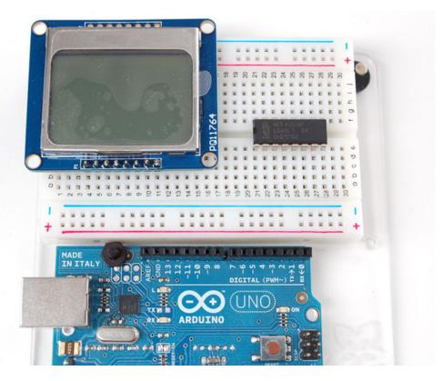
We'll start with the power lines. the system must be powered by 3.3V so red here is connected to the 3V pin from the Arduino. Ground is black.
