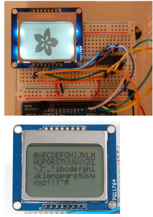
This is a quick tutorial for our 84x48 pixel monochrome LCD display. These displays are small, only about 1.5" diameter, but very readable due and comes with a backlight. This display is made of 84x48 individual pixels, so you can use it for graphics, text or bitmaps. These displays are inexpensive, easy to use, require only a few digital I/O pins and are fairly low power as well.
