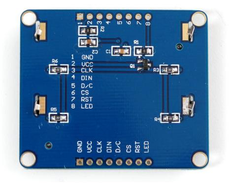
If you want to use the backlight, that can draw up to 80mA (4 white LEDs at 20mA each). The backlight pin is connected to a transistor so you can PWM all 4 LEDs at once from a microcontroller pin.
