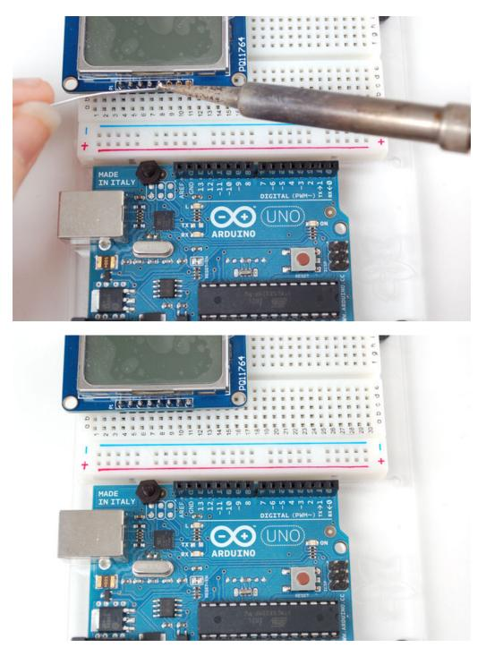
Place the level shifter chip off to the side. Pin 1 is on the left here.
