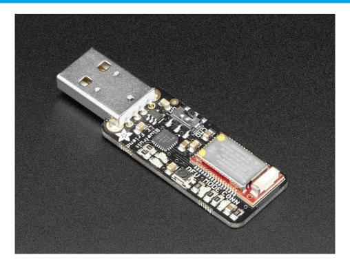
In it's simplest form, it works on the same principle as a common USB/Serial adapter (the FTDI Friend (https://adafru.it/dQa), for example!). Any data that you enter via your favorite terminal emulator on your development machine will be transferred over the air to the connected phone or tablet, and vice versa.
