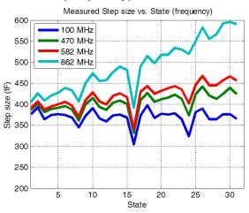
Figure 8. Measured Shunt C vs Frequency (major states)
