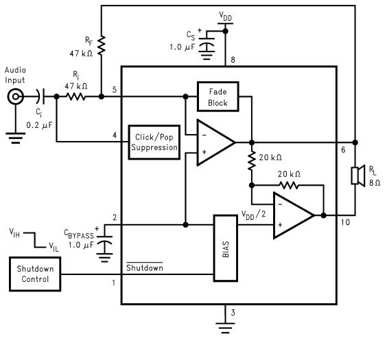
Figure 2. Typical Audio Amplifier Application Circuit
