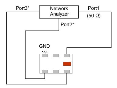
\*Impedance for ports 2 and 3=1/2(Balanced impedance)
